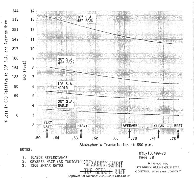
respectively (a CORN tri-bar target) is illuminated under various conditions and is acquired from various scan (roll) angles.
